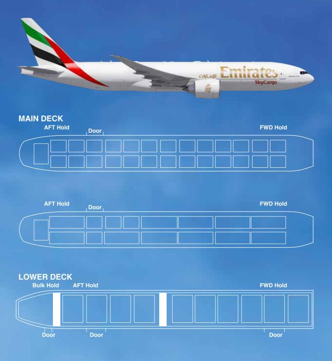
The Boeing 777F is the most environmentally-friendly freighter operated today, with the lowest fuel burn of any comparably-sized cargo aircraft. Along with its wide-deck cargo door which can accomodate oversized consignments, it is also capable of carrying up to 103 tonnes of cargo non-stop on -10hour sector lengths.
