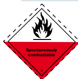
Hazard label for class 4 - Substances Liable to Spontaneous Combustion (Divisions 4.2)
